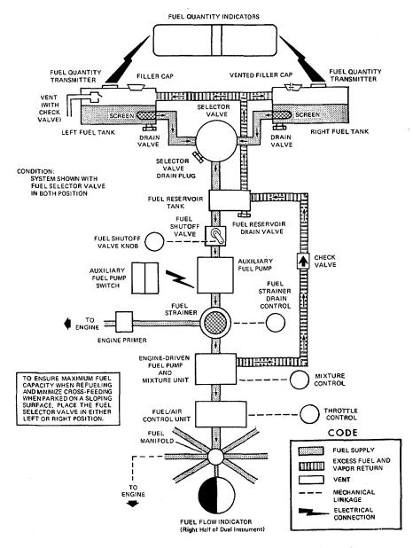
Figure 7-5. Fuel System (Standard and Long Range)
