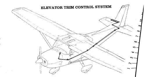
Figure 7-1. Flight Control and Trim Systems (Sheet
