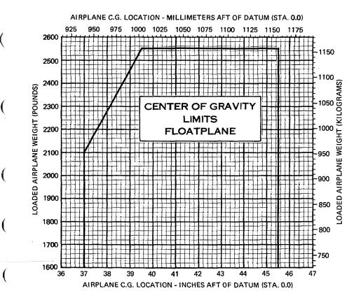
Figure 14. Center of Gravity Limits
