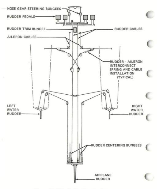
Figure 16. Water Rudder Steering System
