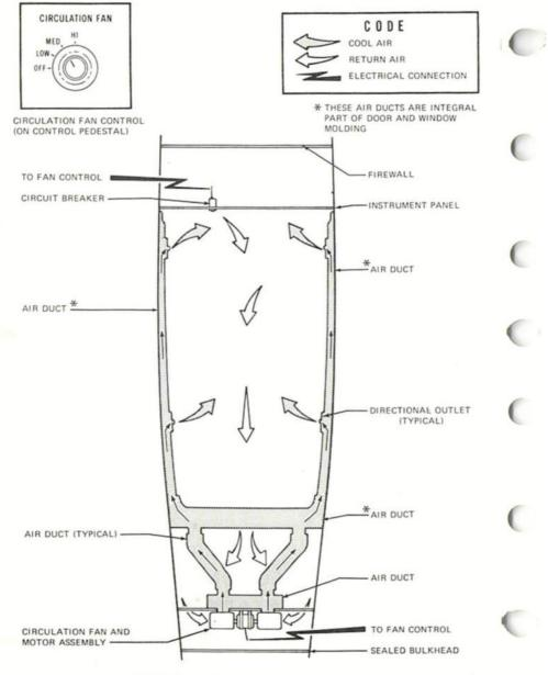
Figure 1. Circulation Fan System
