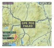
Figure 3 GPS POS FAILED indication
