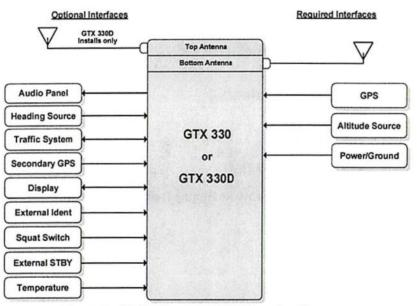
Figure 1 - GTX 330 or GTX 330D Interface Summary
