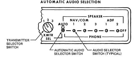
As illustrated, the number 1 transmitter is selected, the AUTO selector switch is in the SPEAKER position, and the NAV/COM 1, 2 and 3 and ADF 1 and 2 audio selector switches are in the OFF position. With the switches set as shown, the pilot will transmit on the number 1 transmitter and hear the number 1 NAV/COM receiver through the airplane speaker.
