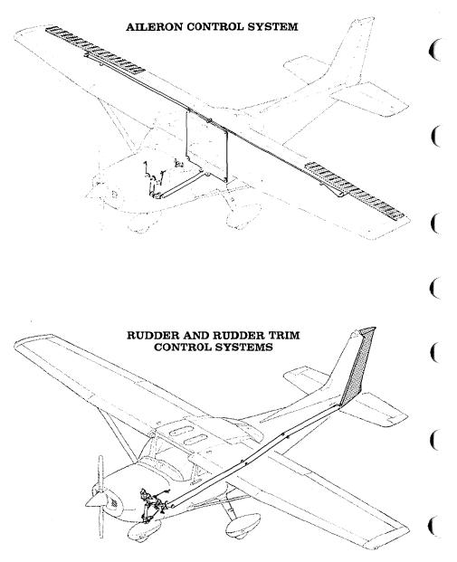
Figure 7-1. Flight Control and Trim Systems (Sheet 1 of 2)
